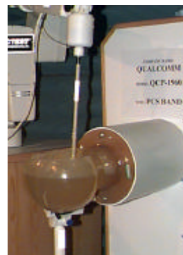
Figure 1. SAR Test Set-up
