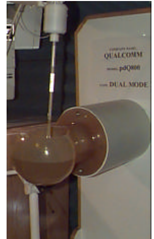
Fig 1. SAR Test Set-up
