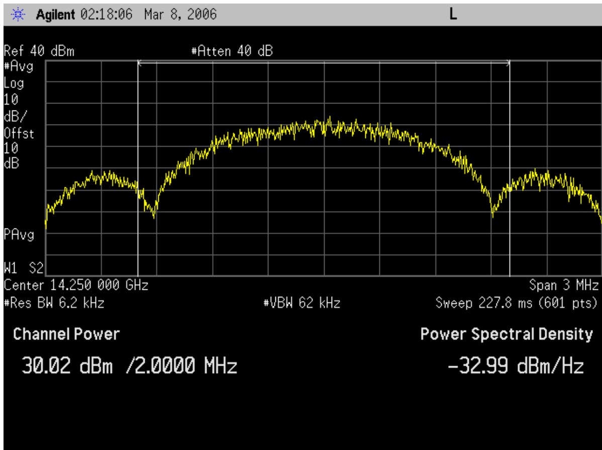
Figure D-3. Conducted RF power from antenna flange, mid band
