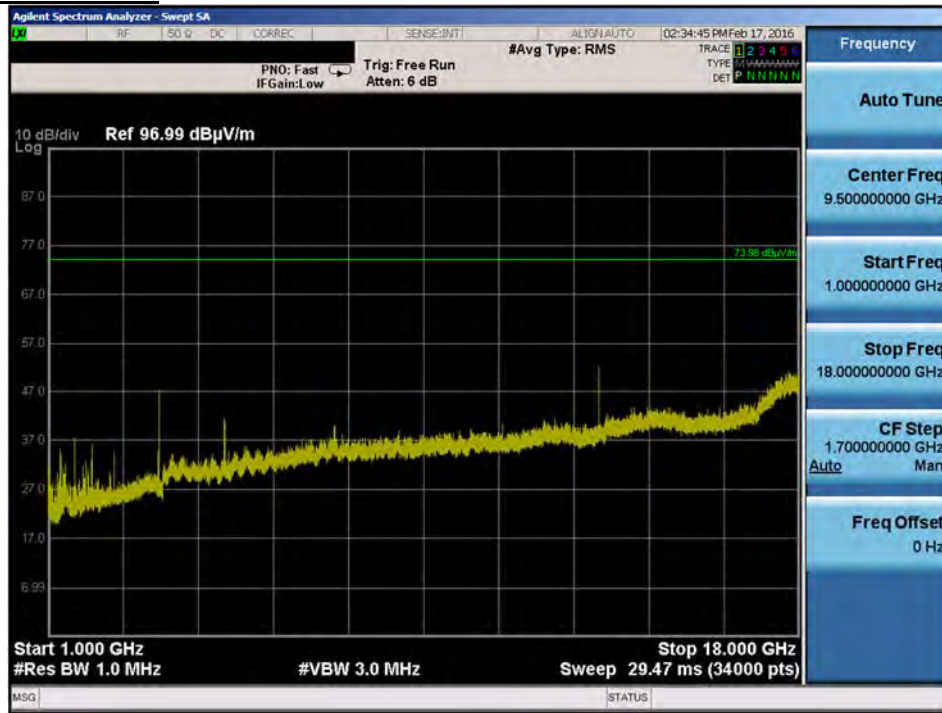
Plot 7-185. Radiated Spurious Plot > 1GHz (LAA (UNII Band 1, 20MHz BW), Ch. 47290)
