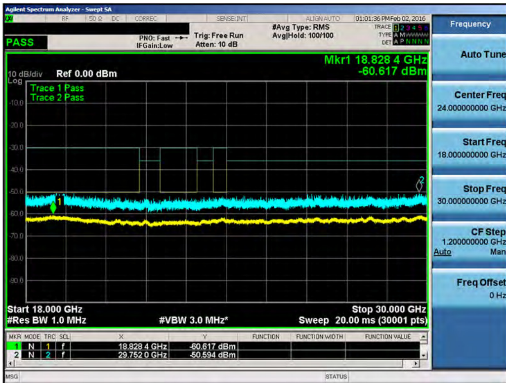
Plot 7-136. Conducted Spurious Plot (LAA (UNII Band 1, 40MHz BW) – Ch. 47290, 47490)
