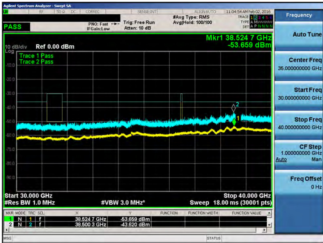
Plot 7-162. Conducted Spurious Plot (LAA (UNII Band 3, 40MHz BW) – Ch. 52740, 52940)
