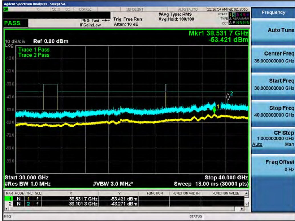
Plot 7-167. Conducted Spurious Plot (LAA (UNII Band 3, 40MHz BW) – Ch. 53140, 53340)
