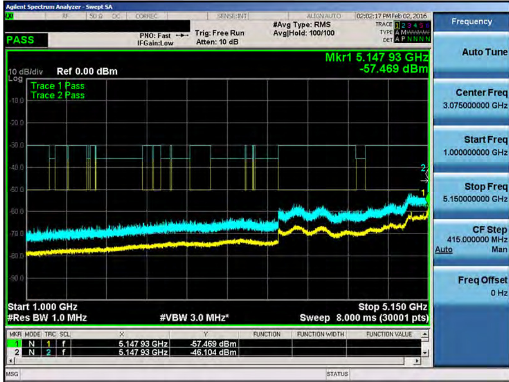
Plot 7-139. Conducted Spurious Plot (LAA (UNII Band 1, 40MHz BW) – Ch. 47490, 47690)
