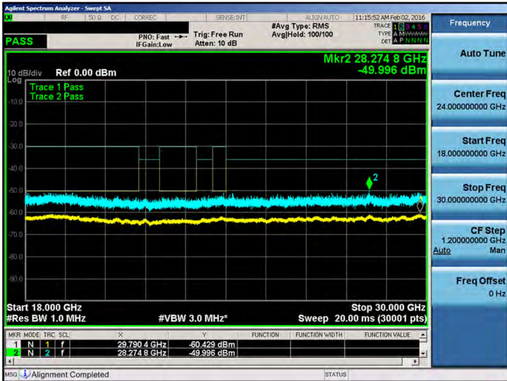
Plot 7-166. Conducted Spurious Plot (LAA (UNII Band 3, 40MHz BW) – Ch. 53140, 53340)
