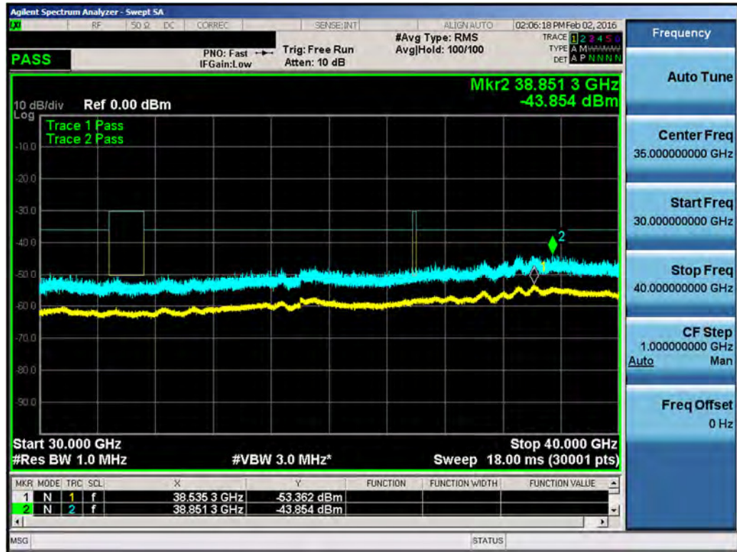
Plot 7-142. Conducted Spurious Plot (LAA (UNII Band 1, 40MHz BW) – Ch. 47490, 47690)
