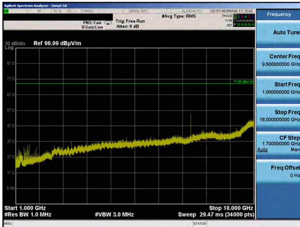
Plot 7-174. Radiated Spurious Plot > 1GHz (LAA (UNII Band 3, 20MHz BW), Ch. 53140)
