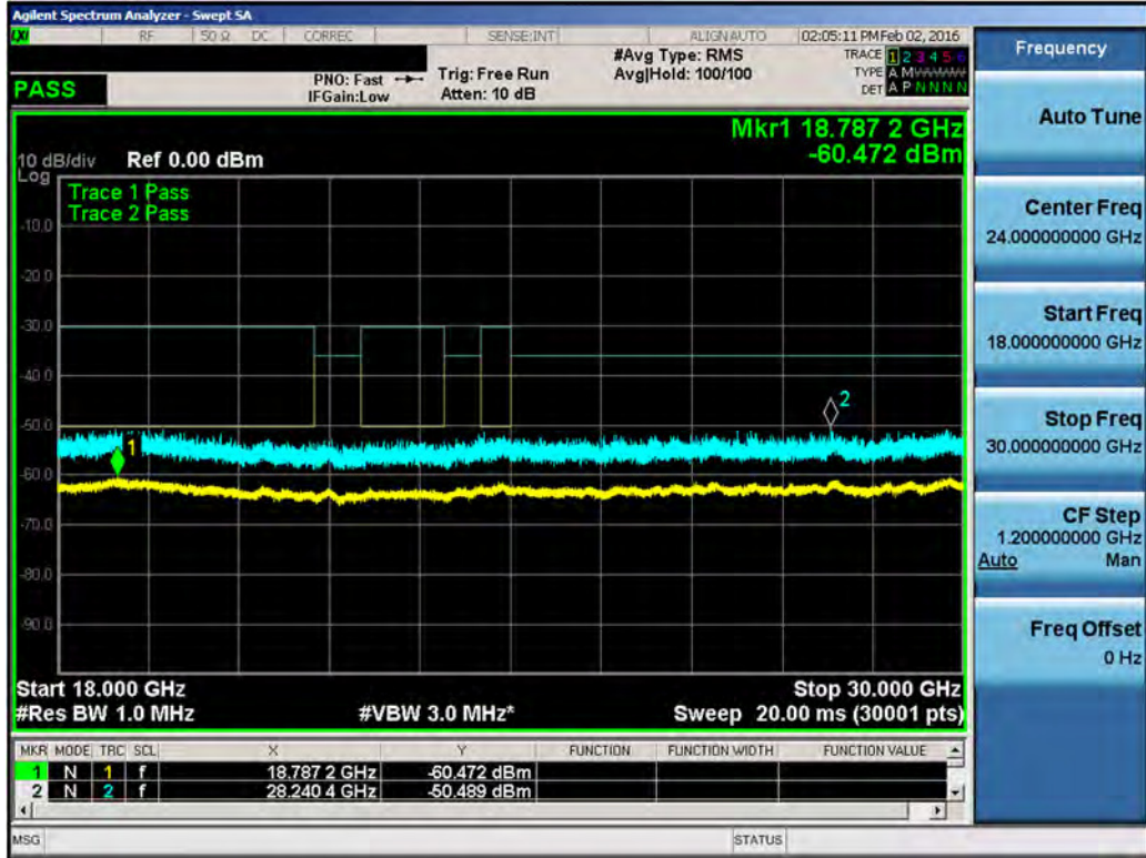
Plot 7-141. Conducted Spurious Plot (LAA (UNII Band 1, 40MHz BW) – Ch. 47490, 47690)
