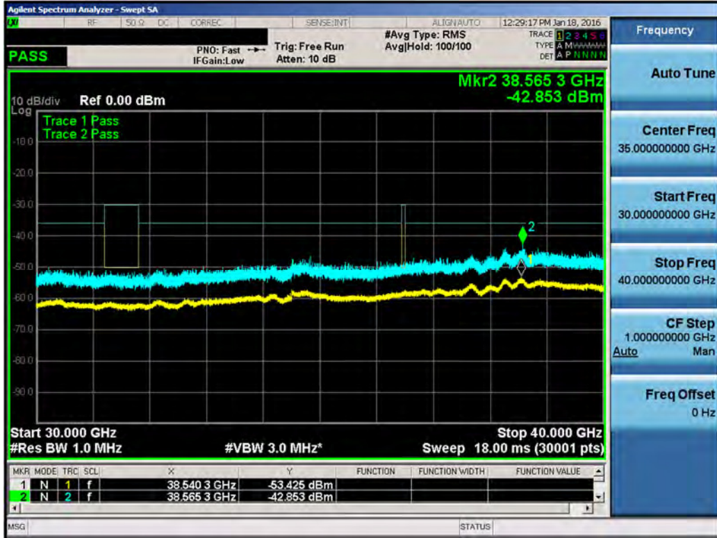
Plot 7-147. Conducted Spurious Plot (LAA (UNII Band 3, 20MHz BW) – Ch. 52740)
