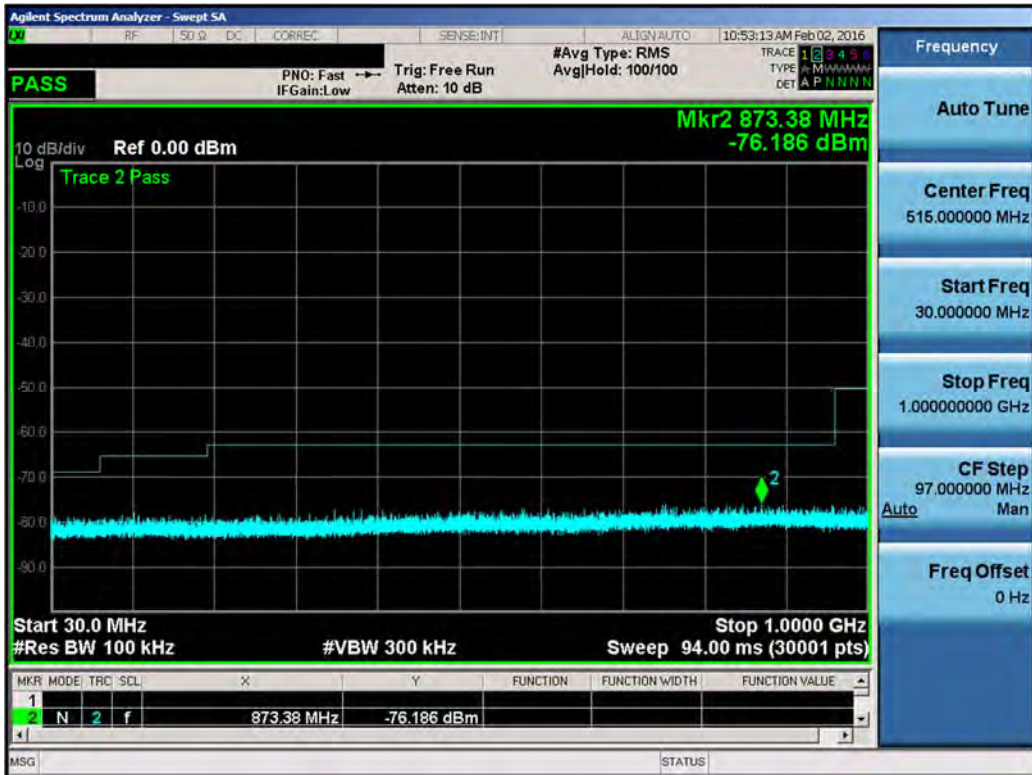
Plot 7-158. Conducted Spurious Plot (LAA (UNII Band 3, 40MHz BW) – Ch. 52740, 52940)
