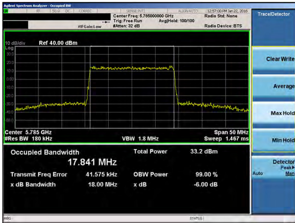
Plot 7-3. 6dB Bandwidth Plot (LAA (UNII Band 3, 20MHz BW) – Ch. 53140)
