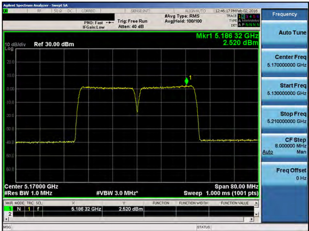
Plot 7-20. Power Spectral Density Plot (LAA (UNII Band 1, 40MHz BW) – Ch. 46890, 47090)
