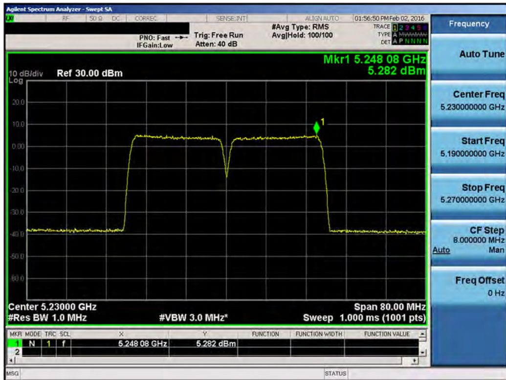
Plot 7-22. Power Spectral Density Plot (LAA (UNII Band 1, 40MHz BW) – Ch. 47490, 47690)
