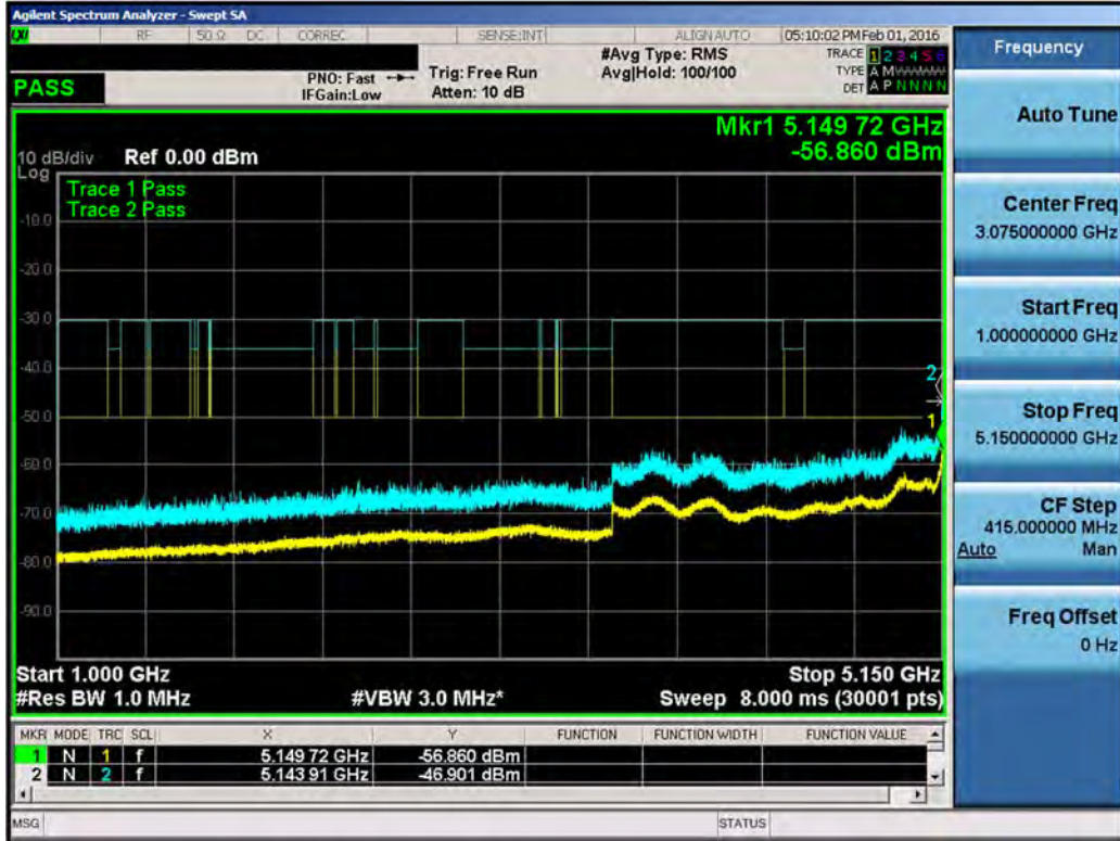
Plot 7-79. Conducted Spurious Plot (LAA (UNII Band 1, 40MHz BW) – Ch. 47490, 47690)
