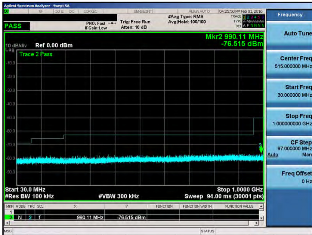
Plot 7-68. Conducted Spurious Plot (LAA (UNII Band 1, 40MHz BW) – Ch. 46890, 4790)
