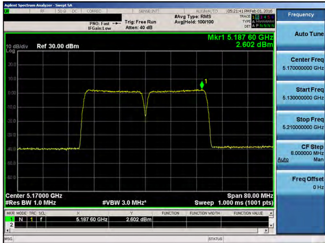
Plot 7-8. Power Spectral Density Plot (LAA (UNII Band 1, 40MHz BW) – Ch. 46890, 47090)
