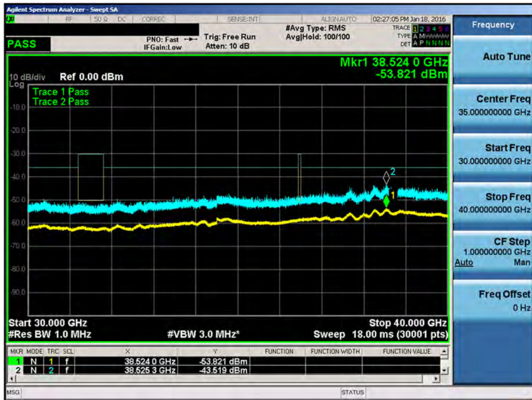
Plot 7-62. Conducted Spurious Plot (LAA (UNII Band 1, 20MHz BW) – Ch. 47290)
