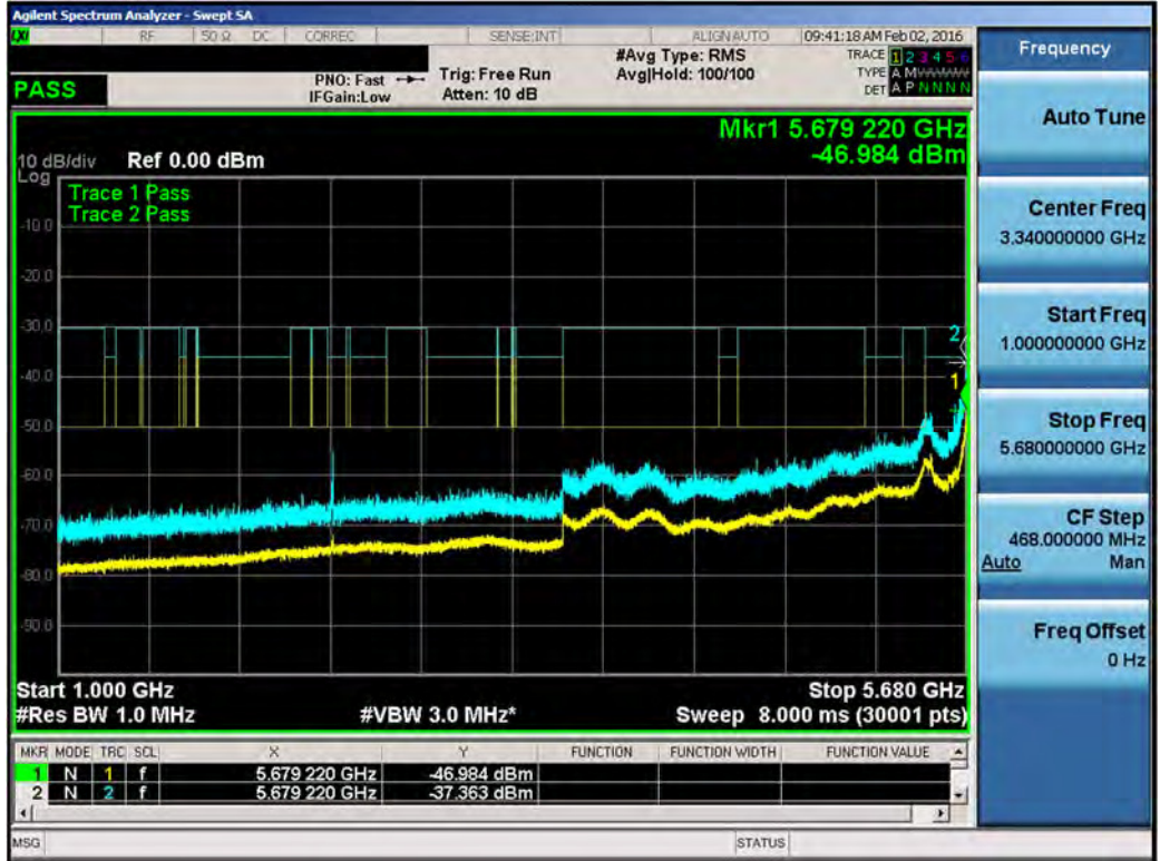
Plot 7-99. Conducted Spurious Plot (LAA (UNII Band 3, 40MHz BW) – Ch. 52740, 52940)
