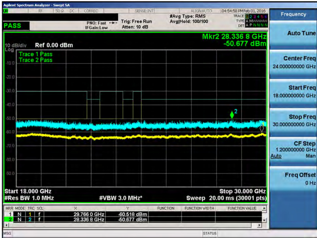
Plot 7-76. Conducted Spurious Plot (LAA (UNII Band 1, 40MHz BW) – Ch. 47290, 47490)
