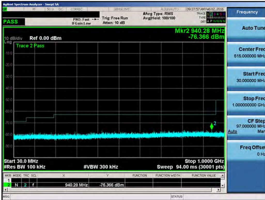
Plot 7-98. Conducted Spurious Plot (LAA (UNII Band 3, 40MHz BW) – Ch. 52740, 52940)
