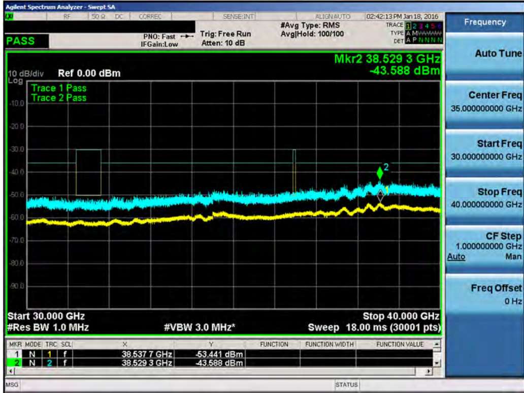
Plot 7-67. Conducted Spurious Plot (LAA (UNII Band 1, 20MHz BW) – Ch. 47690)
