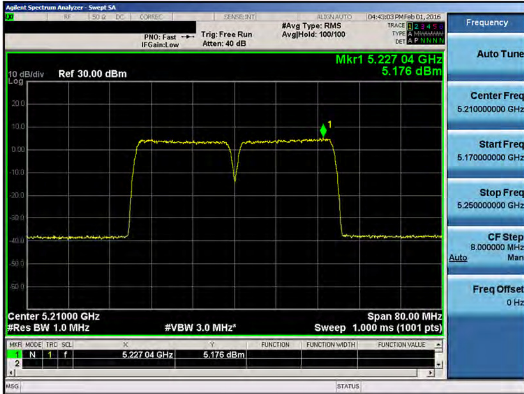
Plot 7-9. Power Spectral Density Plot (LAA (UNII Band 1, 40MHz BW) – Ch. 47290, 47490)
