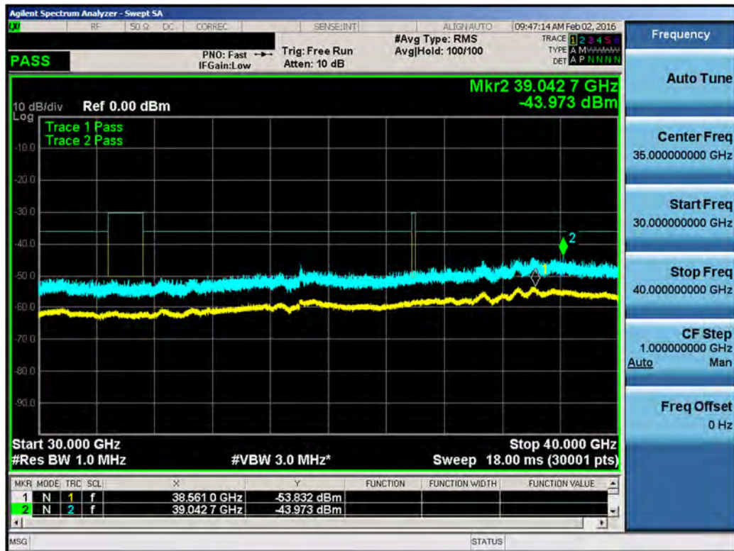
Plot 7-102. Conducted Spurious Plot (LAA (UNII Band 3, 40MHz BW) – Ch. 52740, 52940)
