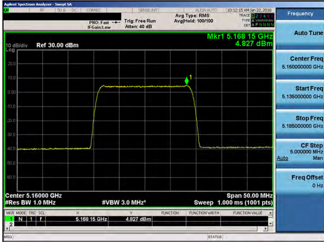
Plot 7-17. Power Spectral Density Plot (LAA (UNII Band 1, 20MHz BW) – Ch. 46890)
