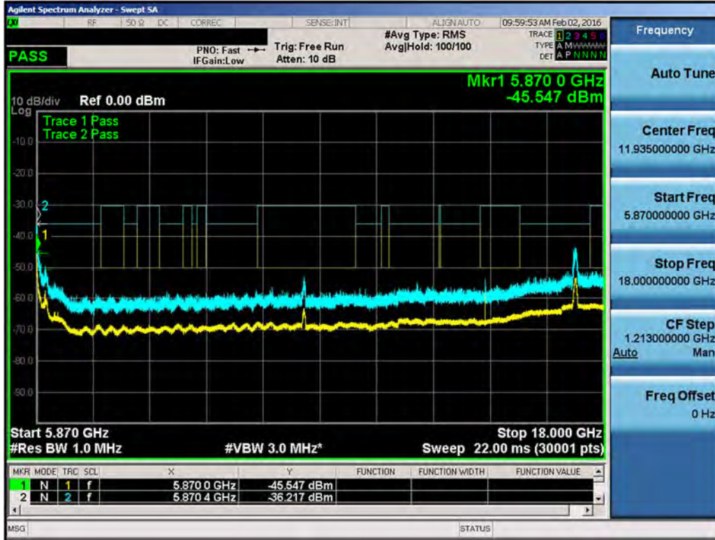
Plot 7-105. Conducted Spurious Plot (LAA (UNII Band 3, 40MHz BW) – Ch. 53140, 53340)
