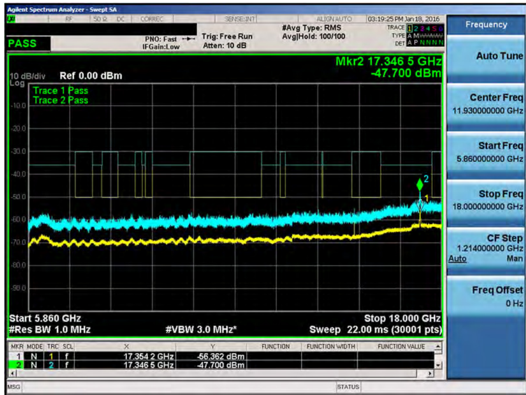
Plot 7-90. Conducted Spurious Plot (LAA (UNII Band 3, 20MHz BW) – Ch. 53140)
