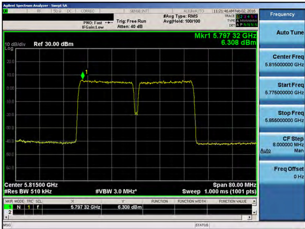
Plot 7-28. Power Spectral Density Plot (LAA (UNII Band 3, 40MHz BW) – Ch. 53340, 53540)
