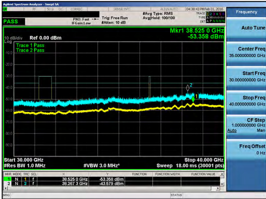
Plot 7-72. Conducted Spurious Plot (LAA (UNII Band 1, 40MHz BW) – Ch. 46890, 47090)
