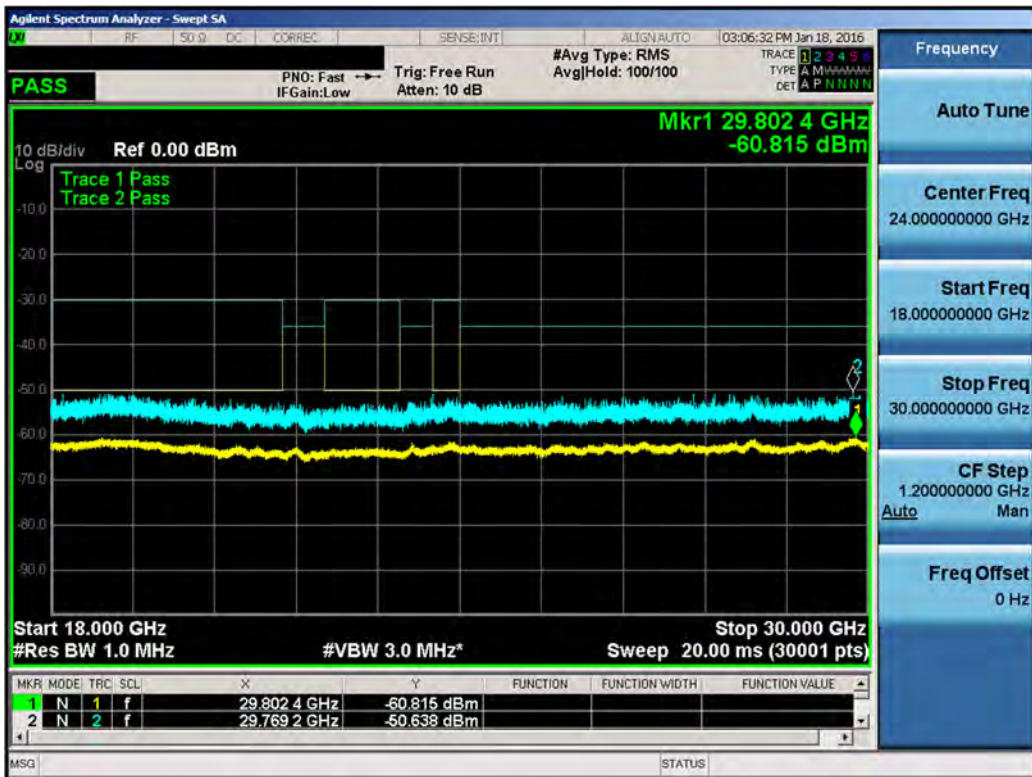
Plot 7-96. Conducted Spurious Plot (LAA (UNII Band 3, 20MHz BW) – Ch. 53540)
