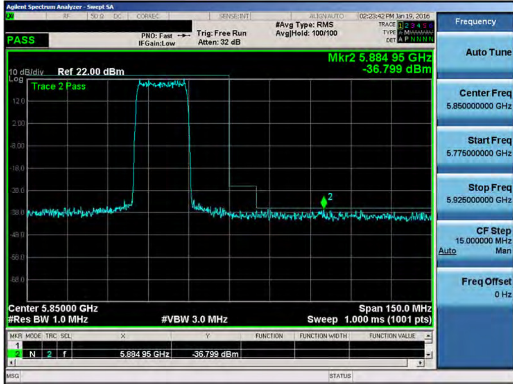
Plot 7-37. Conducted Peak Band Edge Plot (LAA (UNII Band 3, 20MHz BW) – Ch. 53540)
