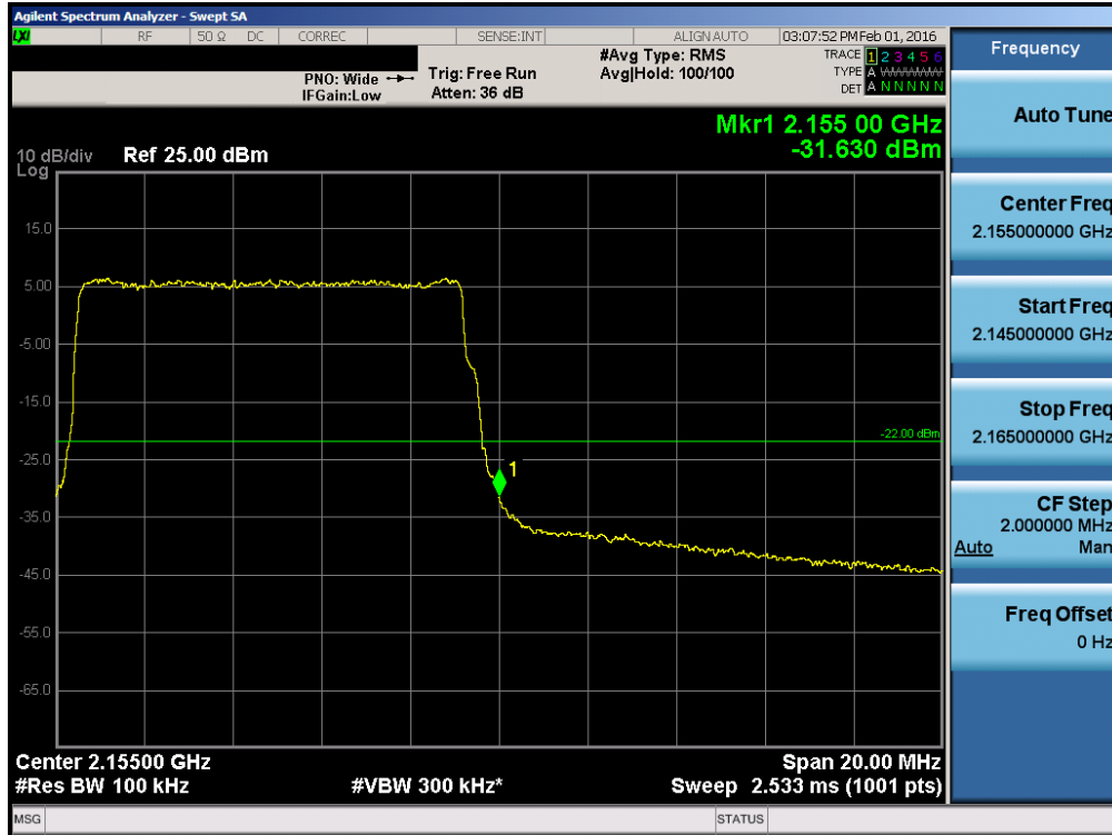
Plot 7-64. Upper Band Edge Plot (Band 4 – 10.0MHz QPSK – RB Size 50)
