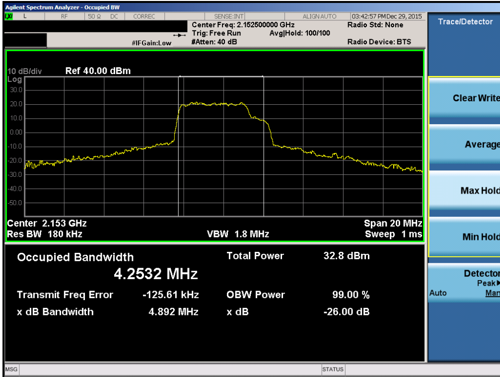
Plot 7-3. Occupied Bandwidth Plot (Band 4 – 5.0MHz QPSK – RB Size 25, High Channel)
