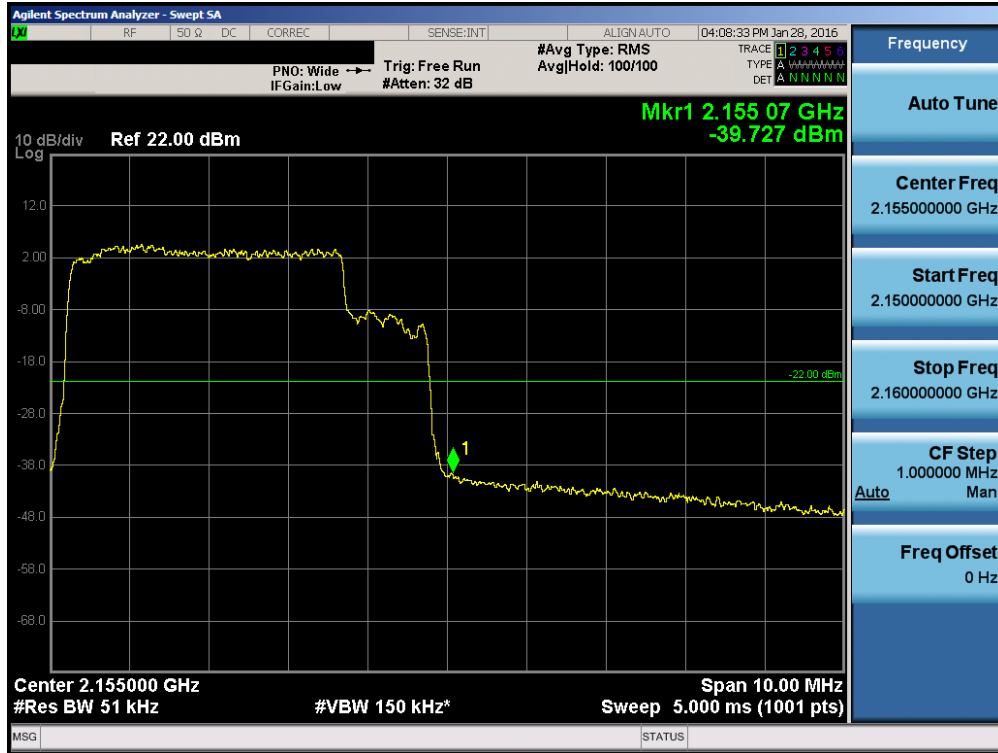
Plot 7-28. Upper Band Edge Plot (Band 4 – 5.0MHz QPSK – RB Size 25)
