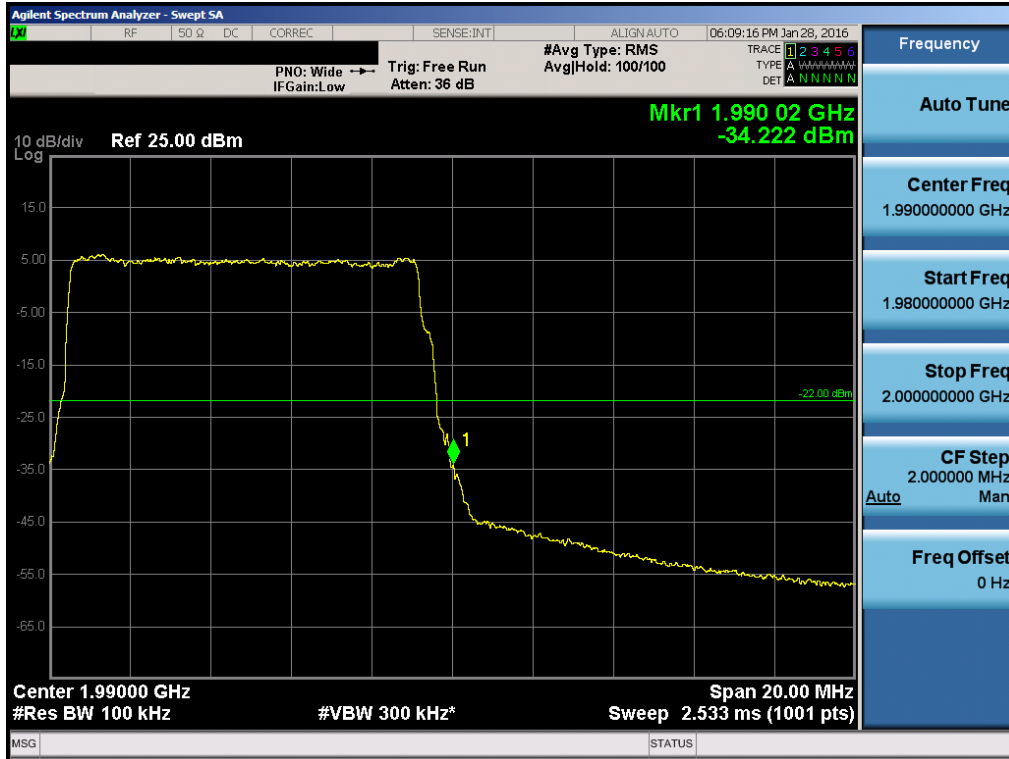
Plot 7-48. Upper Band Edge Plot (Band 2 – 10.0MHz QPSK – RB Size 50)
