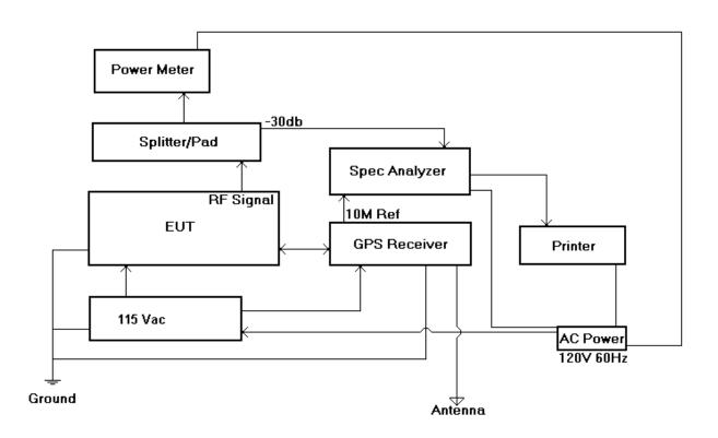
Name of Test:Modulation Characteristics - Frequency Response of Audio<br/>Modulating CircuitParagraph:47 CFR 2.987 (a)Guide:47 CFR 2.987 (a)
