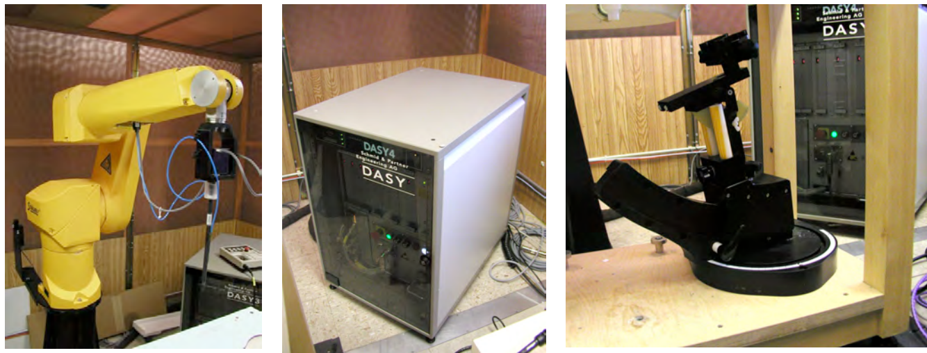
Figure 3-1 DASY4 system: robot arm, controller box, and device positioning holder
