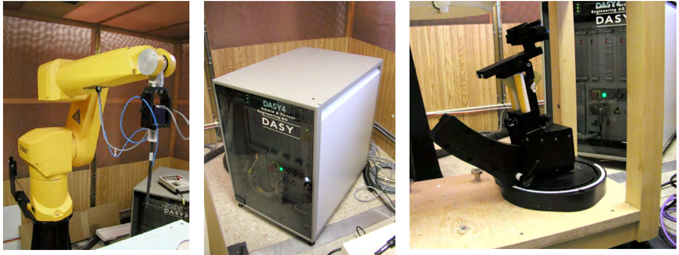
Figure 3-1 DASy4 system: robot arm, controller box, and device positioning holder
