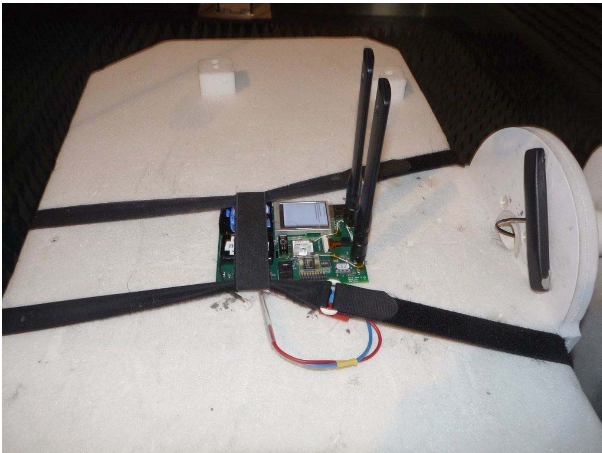
Photo 4: Test setup for radiated measurements (Enclosure, above 1 GHz), detail of EUT setup on tilt device
