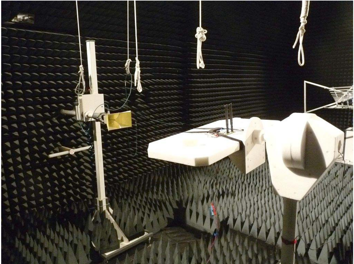
Photo 3: Test setup for radiated measurements (Enclosure, above 1 GHz), EUT and antenna positions
