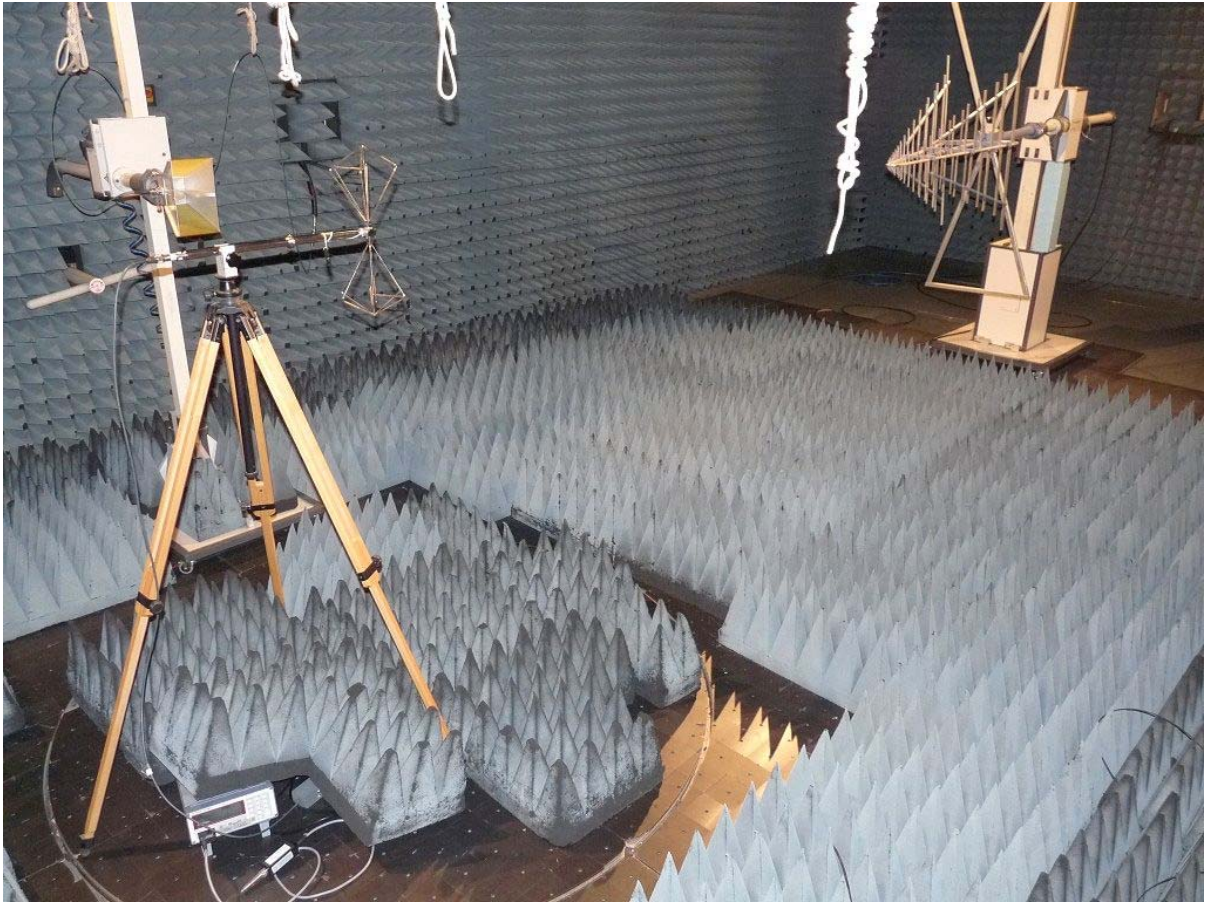
Photo 5: Test setup for substitution measurement (below 1 GHz)
