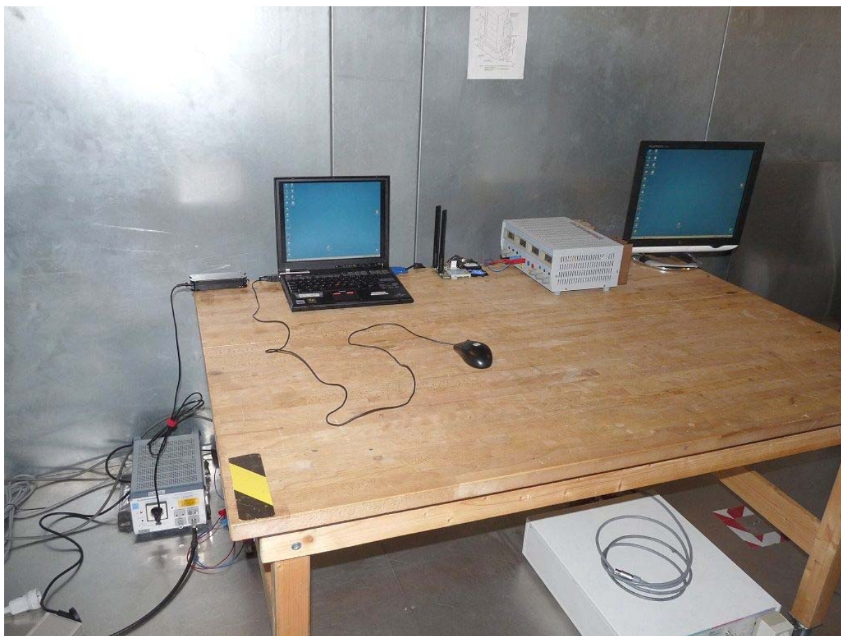
Photo 8: Test setup for conducted measurements (AC Port (power line), computer peripheral setup)
