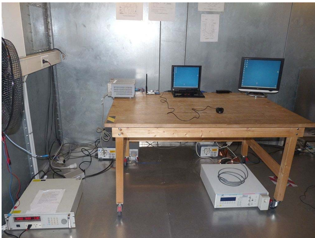
Photo 7: Test setup for conducted measurements (AC Port (power line), powered by external power supply)
