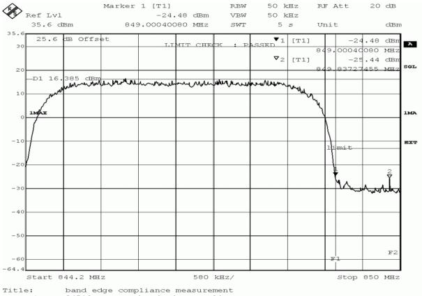
band edge compliance measurement 84510, FDD V, band edge compliance, channel 4233 (846.6MHz) Comment A:
