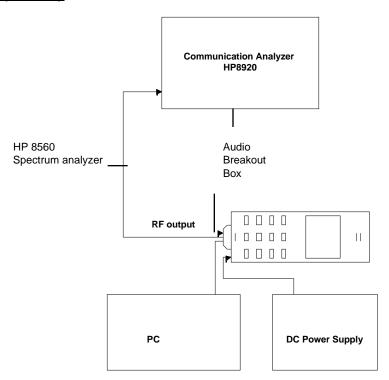
**Definition** - The frequency stability is the ability of the transmitter to maintain an assigned carrier frequency.
