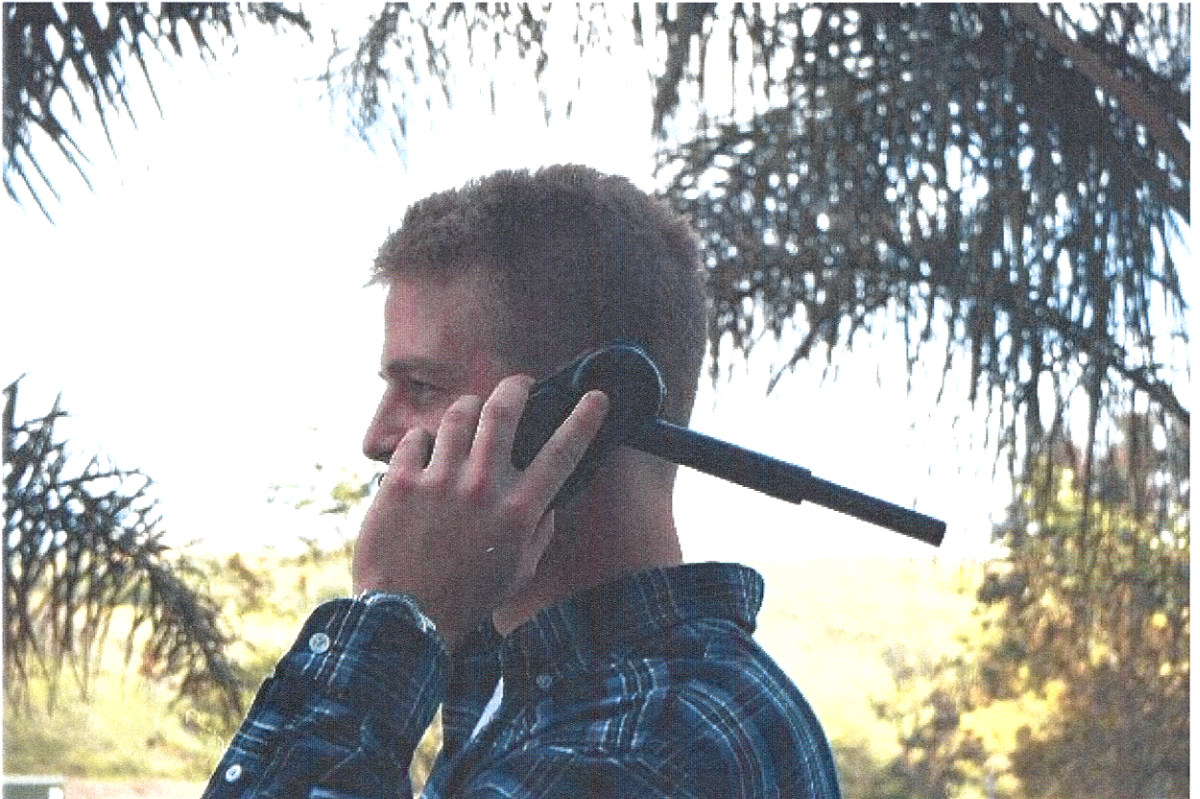
Photo 13 – GSP 1610 With Incorrect Antenna Position
