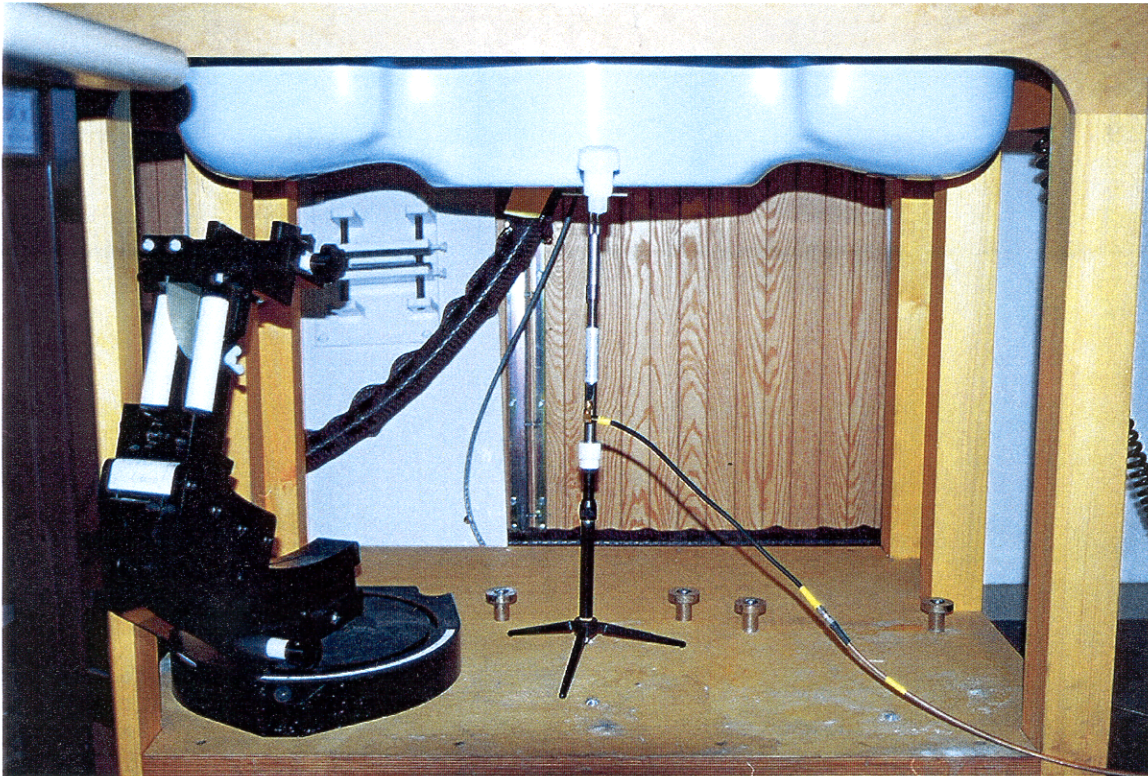
Photo 6 – Validation Dipole Set-up
