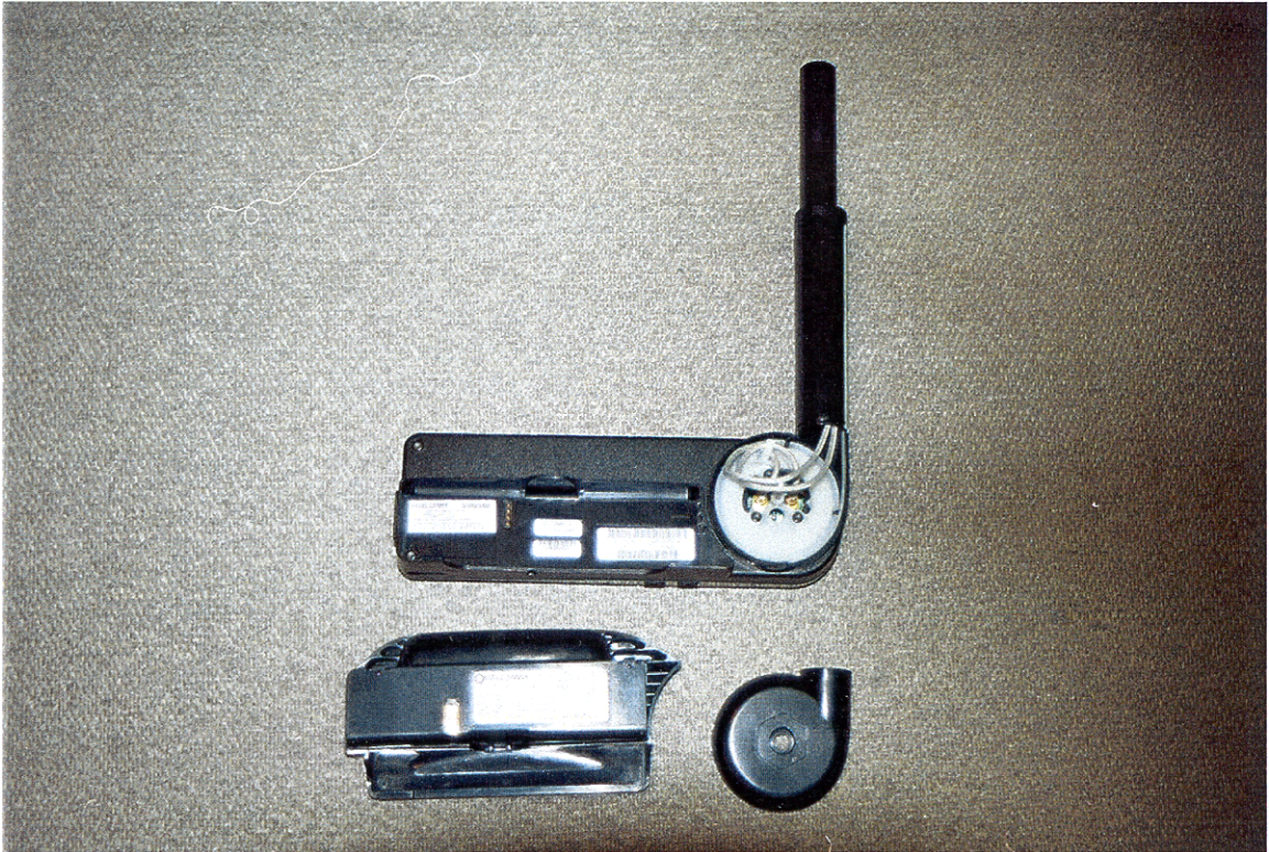
Photo 2 – GSP 1610 Backside with Antenna Cover Removed
