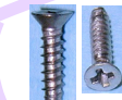
13) Radome Mounting Screws #2 Self Thread Type B 82 Deg. Sheet Metal Screws 18-8 SS 5/16" = 0.314", P/N: SMS505C2R.312 (Item 568)
