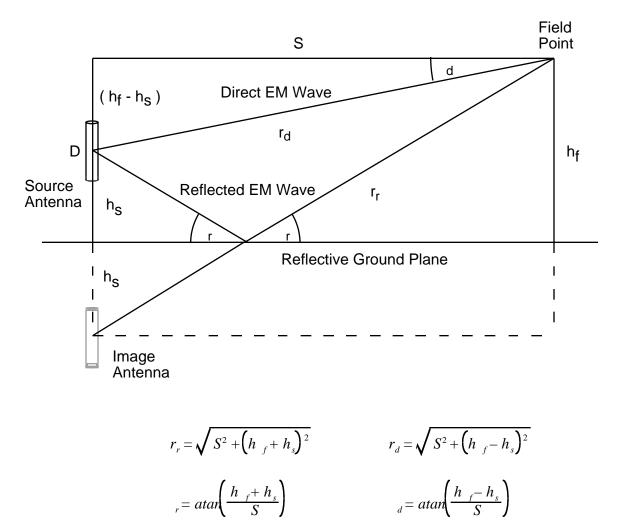
Figure 1. UT MPE Calculation Geometry
