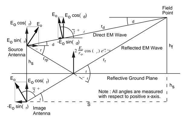
Distance to Ground Plane Reflection Point  $r_{rp} = h_s \csc(r)$
