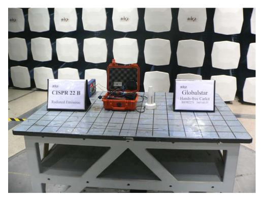
Radiated Receiver Radiated Emissions – Rear View
