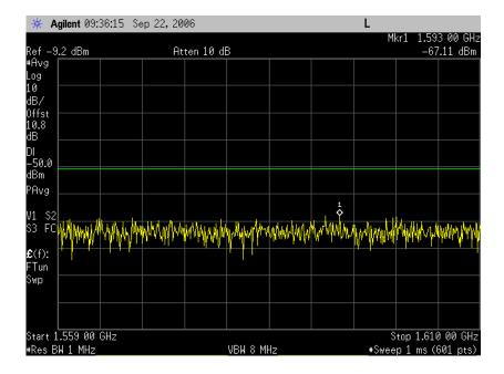
Channel 7 (mid band) carrier off conducted emissions 1559-1610 MHz
