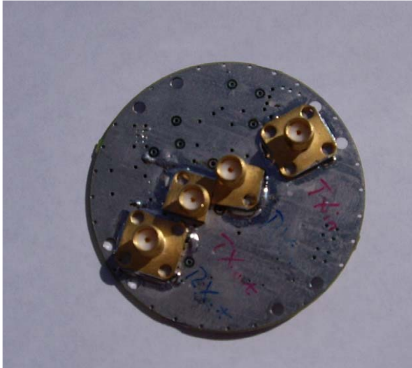
Figure 6 ODU Antenna PCB Top
