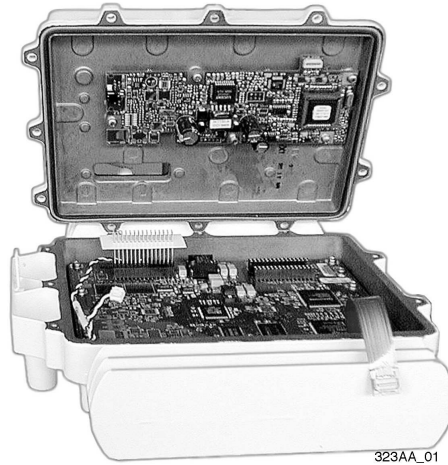
Figure 5. Yellow ribbon and black and white wire disconnected
