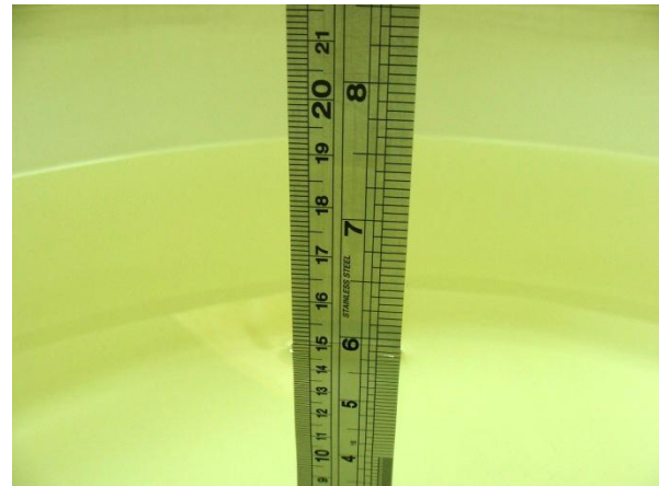
Fig 6.2 Photo of Liquid Height for Body SAR
