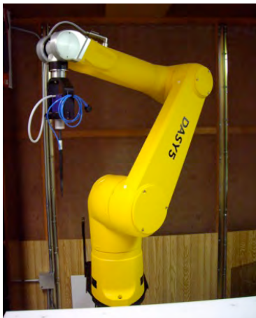
Figure 5-1 DASY5 system: Robot Arm, Controller box, Device Positioning Holder
