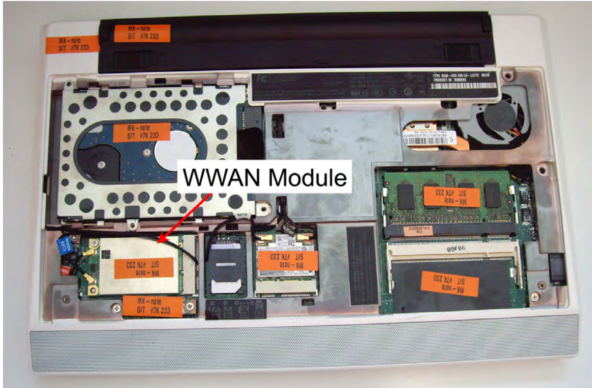
Figure 11-2 Bottom interior view of notebook showing WWAN module location
