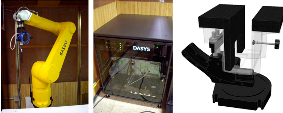
Figure 5-1 DASY5 system: Robot Arm, Controller box, Device Positioning Holder
