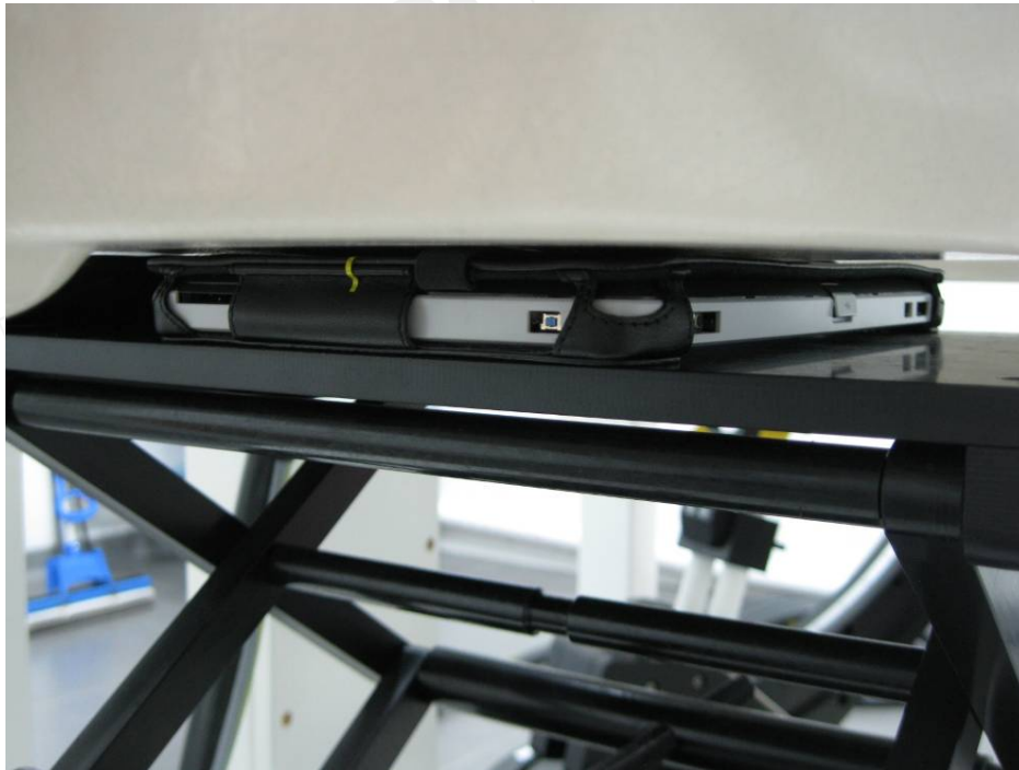
Fig.3 Lap-held mode. ( WWAN/main –to-user separation distance is 12 mm)
