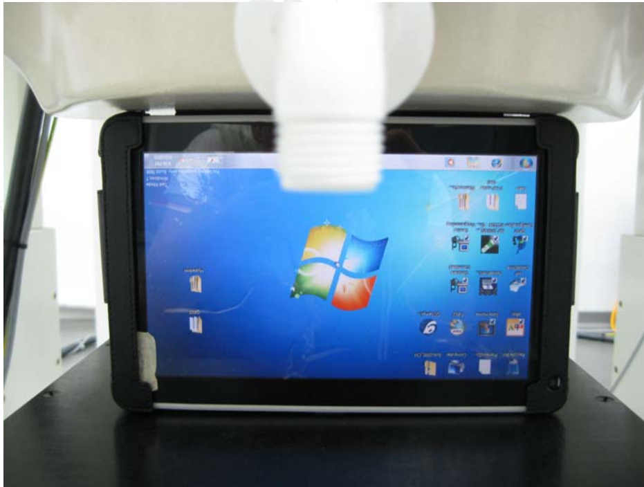
Fig.5 Primary Landscape mode. ( WWAN/main –to-user separation distance is 40 mm)
