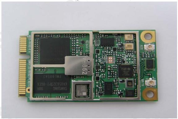
Internal View of EUT -4 (WWAN Module)
