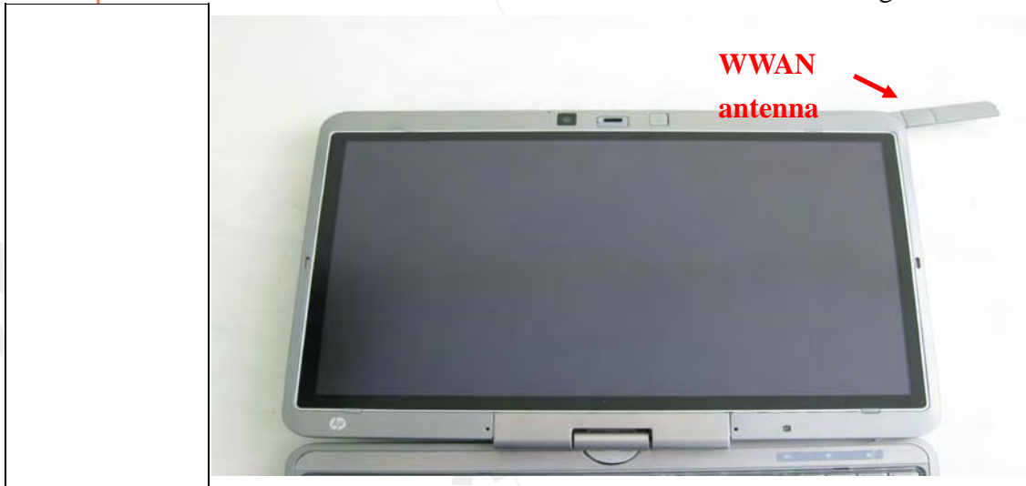
Fig.3 Antenna position of EUT
