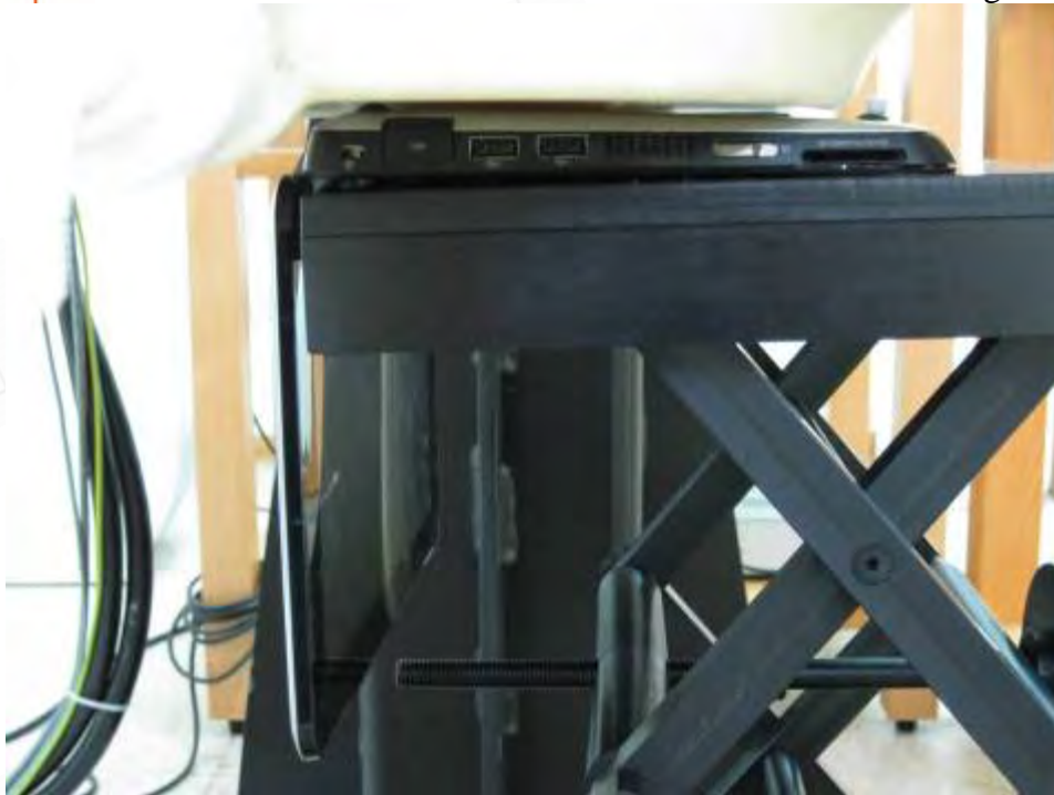
Fig.4 Bottom side of the Notebook is paralleled with flat phantom, open the panel with 90 degrees, bottom side is contact with flat phantom.
