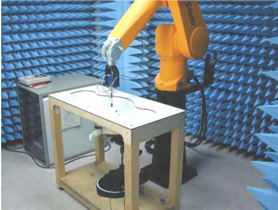
Fig.1 Photograph of the SAR measurement System
