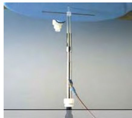
Photograph of the dipole Antenna
