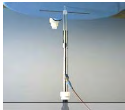
Photograph of the dipole Antenna
