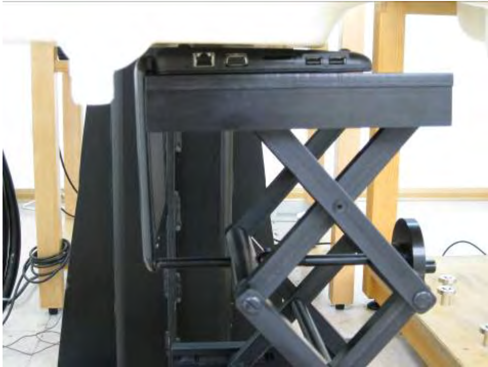
Fig.3 Bottom side of the Notebook is paralleled with flat phantom, open the panel with 90 degrees, bottom side is contact with flat phantom.
