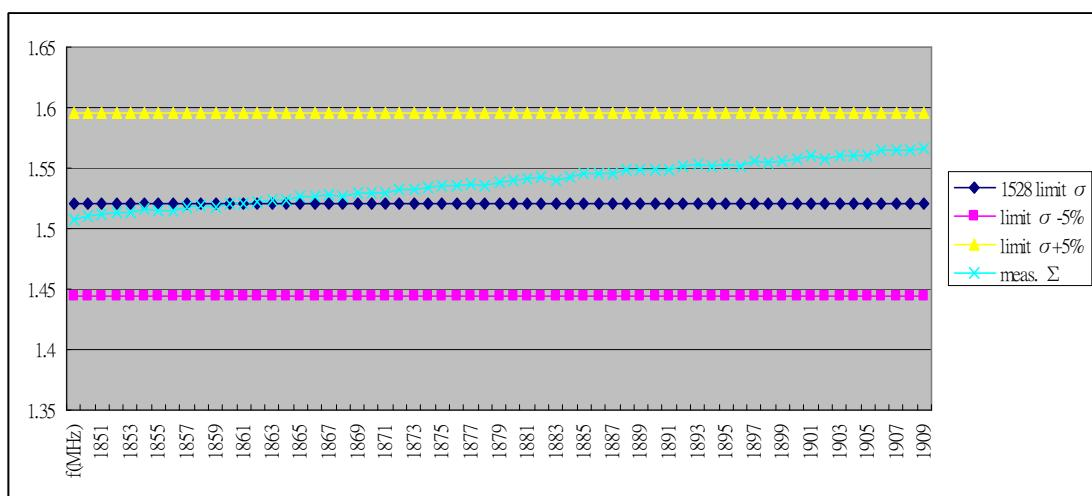
The graphs below show measured permittivity and conductivity values stayed within their respective tolerances of  $\pm 5\%$  of target as required by KDB 450824
