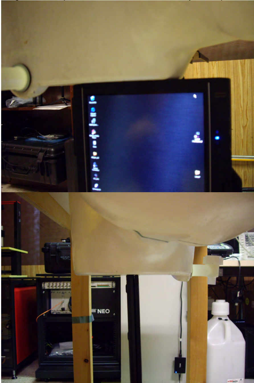
Figure 11-6 DUT positioned under Phantom – Secondary Portrait position
