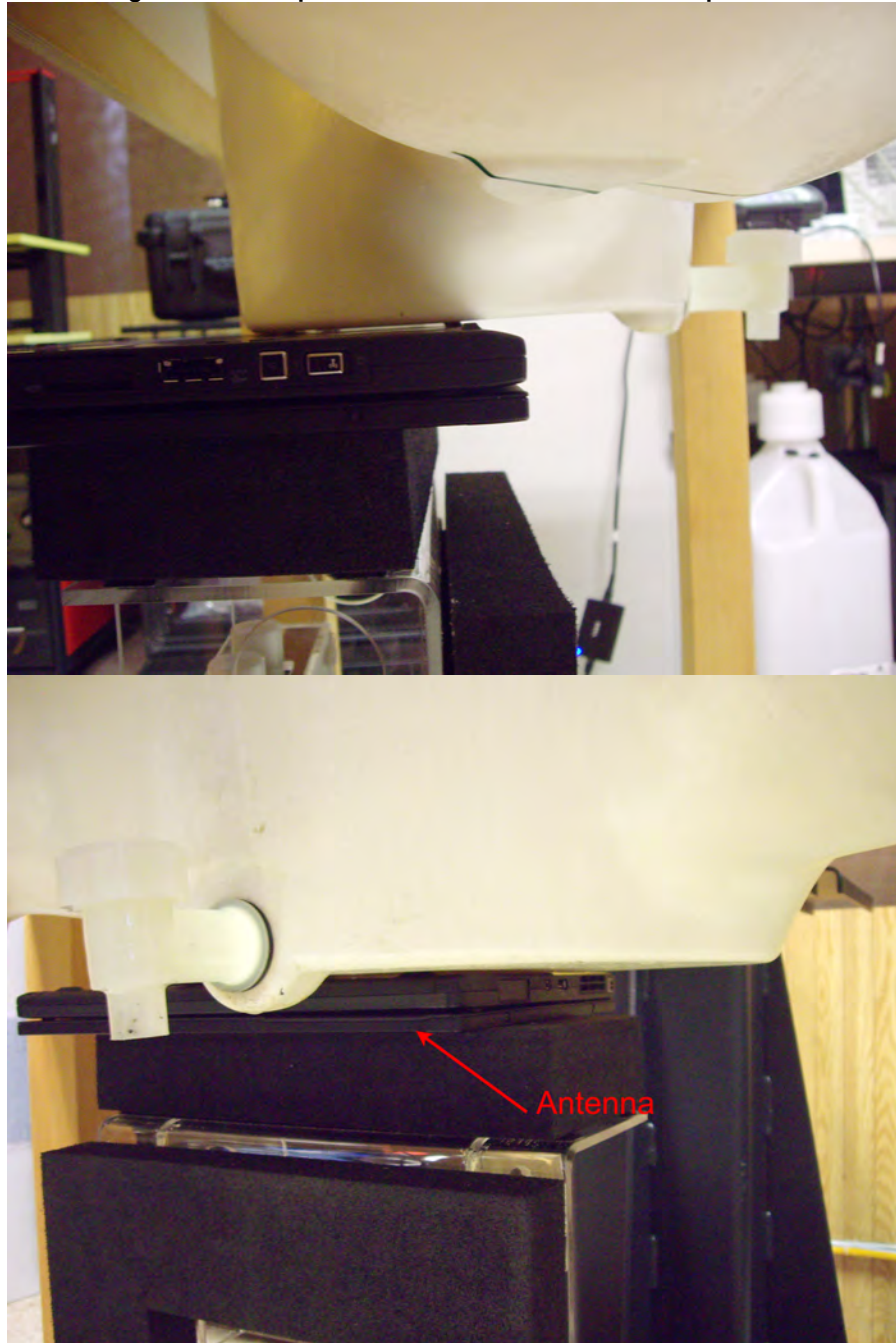
Figure 11-5 DUT positioned under Phantom – Tablet position
