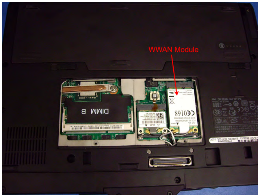
Figure 11-4 Bottom view of notebook showing WWAN module location
