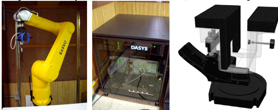
Figure 3-1 DASY5 system: Robot Arm, Controller box, Device Positioning Holder
