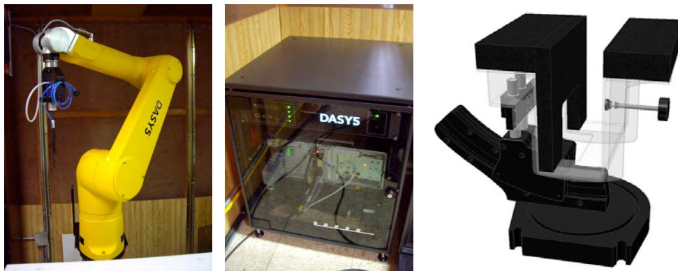
Figure 3-1 DASY5 system: Robot Arm, Controller box, Device Positioning Holder
