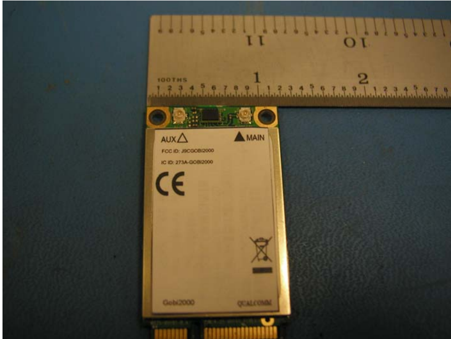
Figure 2 Gobi™2000 Module Rear External Photograph (Shields installed)
