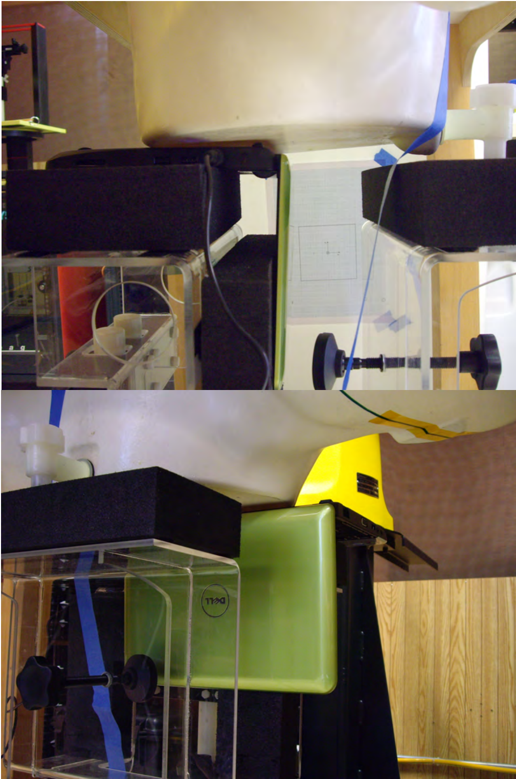
Figure 11-4 Photos of DUT positioned under Phantom
