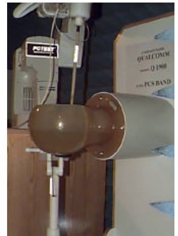
Figure 1. SAR Test Set-up
