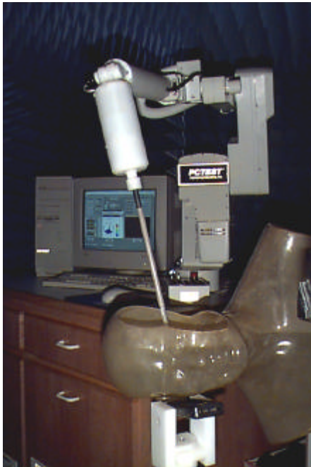
Figure 5. Photograph of the Probe and the Phantom
