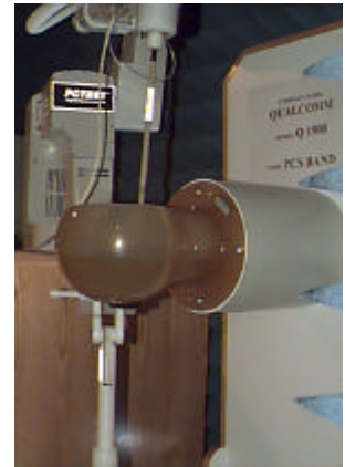
Figure 1. SAR Test Set-up
