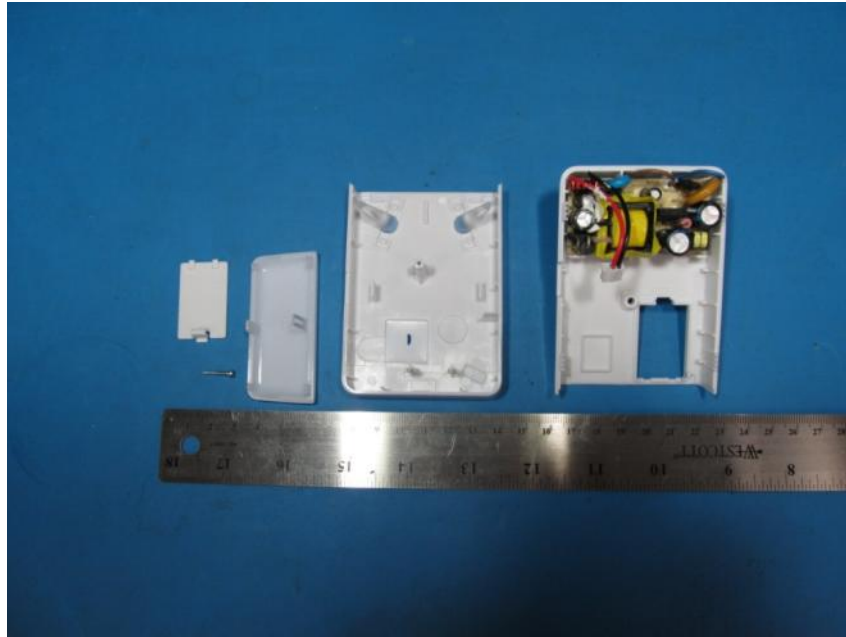
Figure 1-1: Disassembled with only power supply installed
