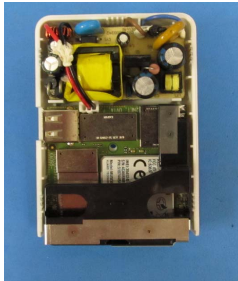
Figure 1-2: Disassembled with power supply and 2net board installed
