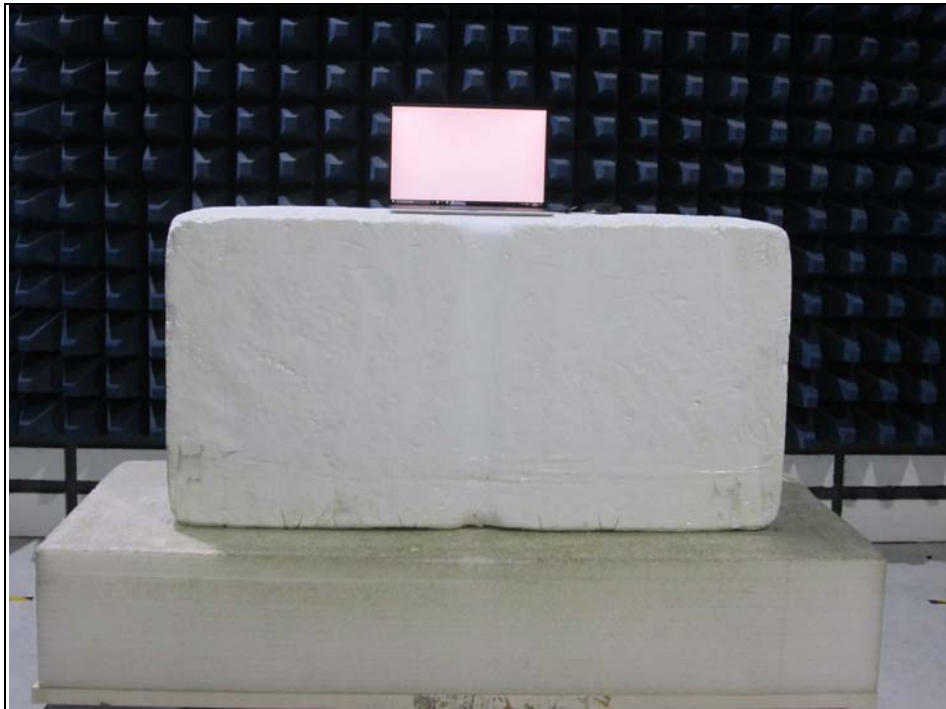
Radiated Emission Test above 1GHz
