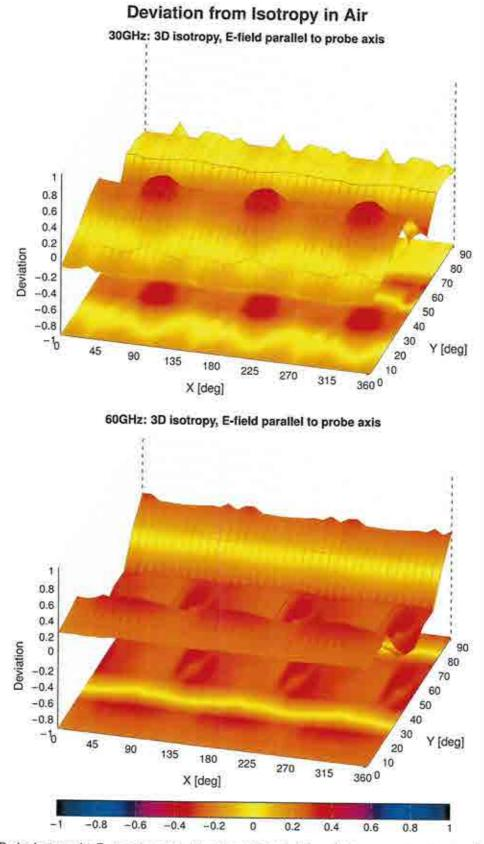
Probe isotropy for E<sub>tot</sub>: probe rotated  $\phi = 0^{\circ}$  to 360°, tilted from field propagation direction  $\vec{k}$ Parallel to the field propagation ( $\psi = 0^{\circ} - 90^{\circ}$ ) at 30 GHz: deviation within ±0.40 dB Parallel to the field propagation ( $\psi = 0^{\circ} - 90^{\circ}$ ) at 60 GHz: deviation within ±0.39 dB
