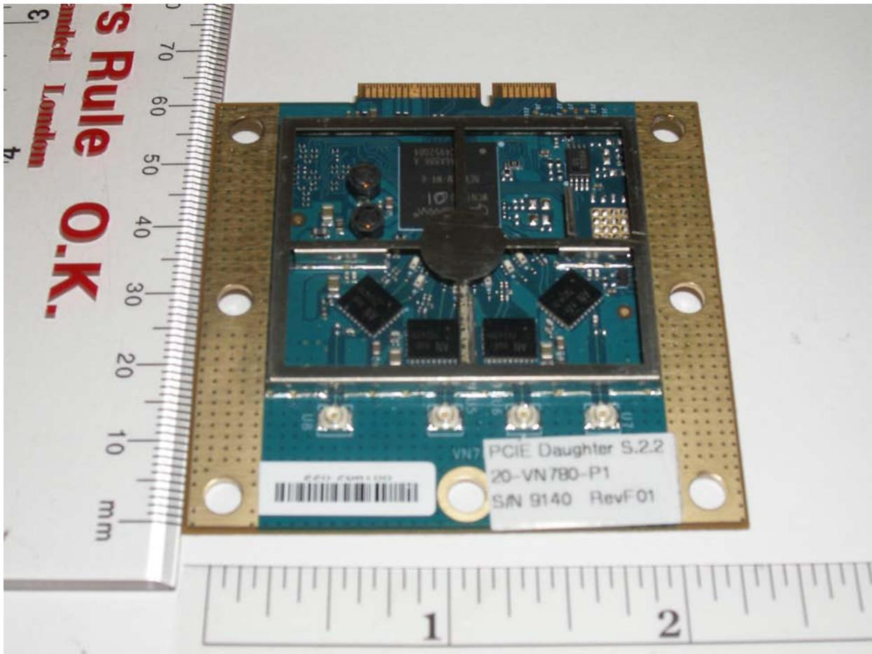
Figure 2 EA544D Family Ethernet Adapter Card without shield(bottom view)
