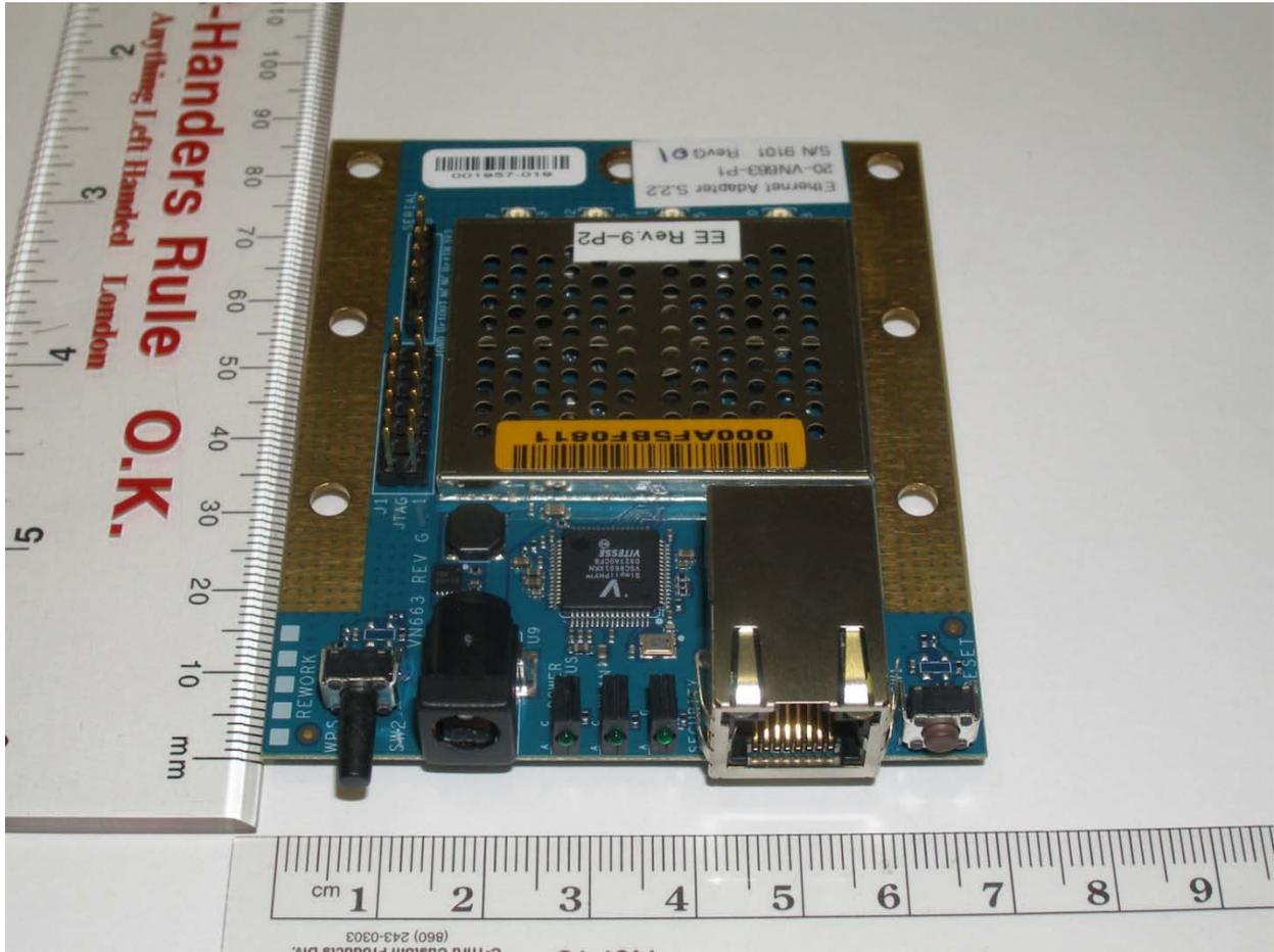
Figure 2 Bottom view of the EA544D Family Ethernet Adapter Card with shield
