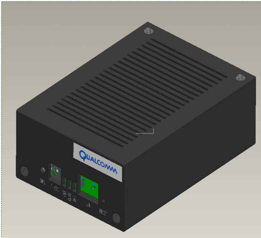
Figure 2-1 Prototype housing with internal EA544D Ethernet adapter
