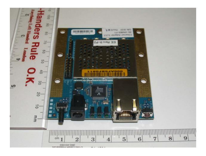
Figure 1 Top view EA544D Family Ethernet Adapter Card with shield
