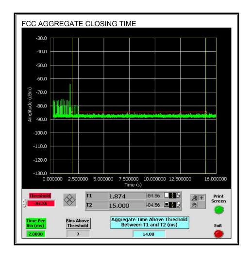
Only intermittent transmissions are observed during the IC aggregate monitoring period.
