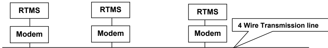
Fig 26. Multi-drop wiring configuration
