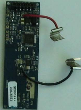
CB942 - battery wires and membrane switch
