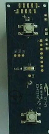
CB960 - battery holder and mechanical switches
