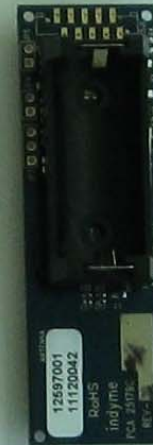
CB960 - battery holder and mechanical switches
